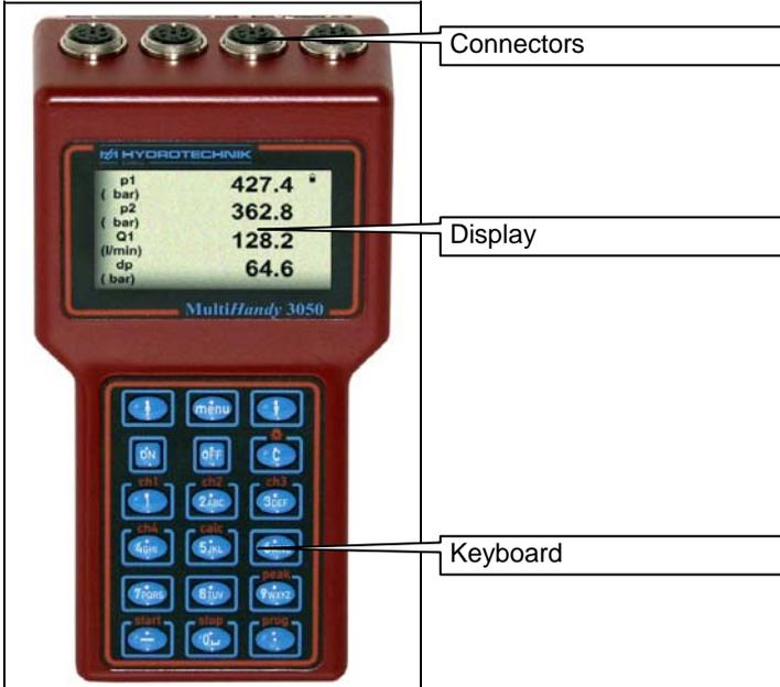
Pic. 1: Components of the measuring instrument
