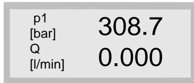
A condition for the measurement of volume flow rate is the connection of a measuring turbine or a gear flow meter with integrated F/DC-converter.
