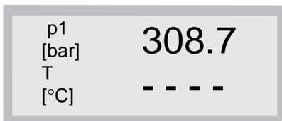
If T (°C) — is displayed, the temperature sensor isn't connected to the measuring instrument. This is only valid for the adjustment of sensor type 4 to 20 mA.
