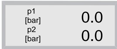
If you request an initialisation, press key o and all data like calibration value, units of measurement, selection of the output signal of the pressure sensors, entered previously, is deleted.
