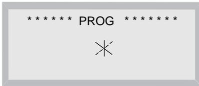
In the display „PROG“ and a rotating bar is shown which indicates, that the selected printer driver is stored in the EEPROM.
