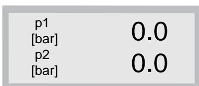
If the pressure sensor works correctly, the measuring value display will be shown in the usual way without horizontal lines.
