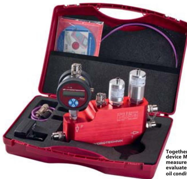
Together with the measuring device MultiSystem 5070, different measurement data can be evaluated and the changes in the oil condition can be displayed.
