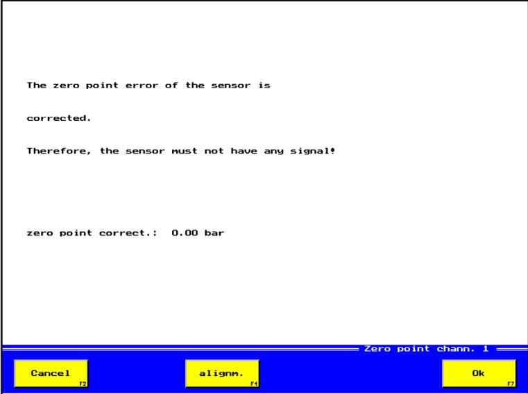
Picture 4.7 Menu: Zero point alignment channel 1
