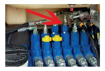
Typical applications include switch speed limitation of excavator booms, excavator bucket movement or the rotation of the cab as well as the optimization of the pre-control of counter-balance valves. The image shows how Minivaly can be integrated in the pre-control line for rotation of the cab of the Volvo Construction Equipment ECR50D mini digger.
