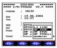
You can choose between HP colour and b/w printers and other makes. The available printers have been tested by HYDROTECHNIK.
