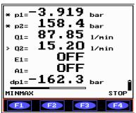
Now all entries have been made and the actual storage is started by pressing which automatically activates the storage menu.
