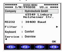
In the line "Company" the company address may be changed to that of the user with the arrow key.
