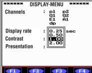
Select the desired display rate with the up/down arrows
