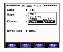
The menu item **Output** also allows the display of statistics and graphics y = f(x) with the key.
