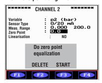
The zero point alignment is set through the option "zero value" with Should, for example, the pressure sensor show a zero value discrepancy although no pressure exists, press (start) to reset the zero value. The zero value discrepancy is stored by the device and later taken into consideration by the software when the actual measure is displayed.
