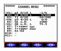
The attached calibration protocol for a pressure sensor provides the necessary calibration points that may be entered line by line as standard or actual values. Please note that each entry must be confirmed with
