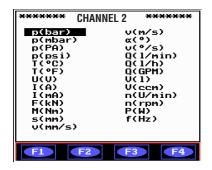
The measuring type is selected with the arrow keys . In our example we select p (bar).
