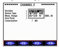
Select "signal type" with [N]. You can only select from 0 to 20 mA, 4 to 20 mA or 0 to 10 V
