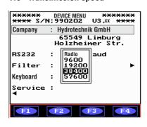
The line "RS 232" lets you select the Baud rate. The desired Baud rate\* is selected with the arrow keys.
