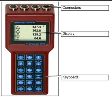
Pic. 1: Components of the measuring instrument
