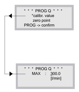
When connecting a volume flow rate sensor (turbine or gear flow meter) to the instrument, the max. volume flow rate needs to be entered as a calibration value.
