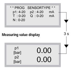
After approx. 3 seconds, the display switches automatically into the measuring value display.
