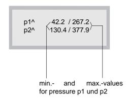
The extreme values (min/max.) can only be shown for the pressure of p1 and p2.
