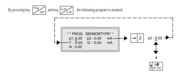
The change-over to 4 to 20 mA is made by a stroke of key  $(p_1-p_2)$ , which is now acting as a cursor and which switches p1 to the
