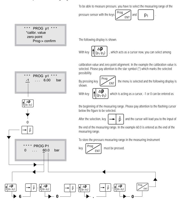
The pressure measuring range for p2 is adjusted in the same way!
