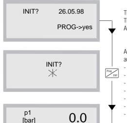
p2 [bar] The display "INIT" is shown for a short period with a rotating bar. This indicates, that the preadjustments are stored in the EEPROM. Afterwards the instrument returns directly into the measuring value display.
