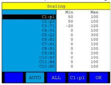
Press [2] to toggle between the input modes "User" (manual input of scaling values) and "Auto".
