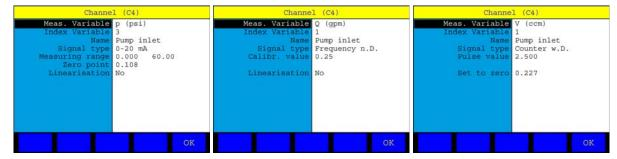
The combined input channels can be used for sensors with analog or frequency output signal. The channel is set by selecting the appropriate signal type.
