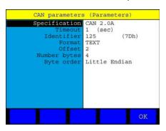
Here you may enter the CAN parameters of the connected sensor or MultiXtend module. The required information can be found in the documentation of the device.
