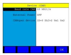
Set the baud rate to the value contained in the Patrick operation menu (here: "125 kBit/s") and enable the CAN bus power supply (External Power "ON").
