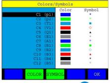
Highlight a channel, press [N], select the desired colors and confirm with [N]; select the desired symbol and confirm with [N]; repeat this for all desired channels.
