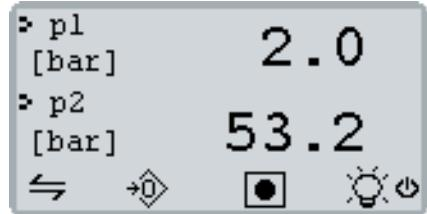
**p1** displays the measurement value of the sensor from channel 1 (**CH1**). Measurement unit **[bar]** follows.
