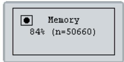
The display automatically switches back after 5 seconds. The measurement series automatically end after 60,000 measurement points.
