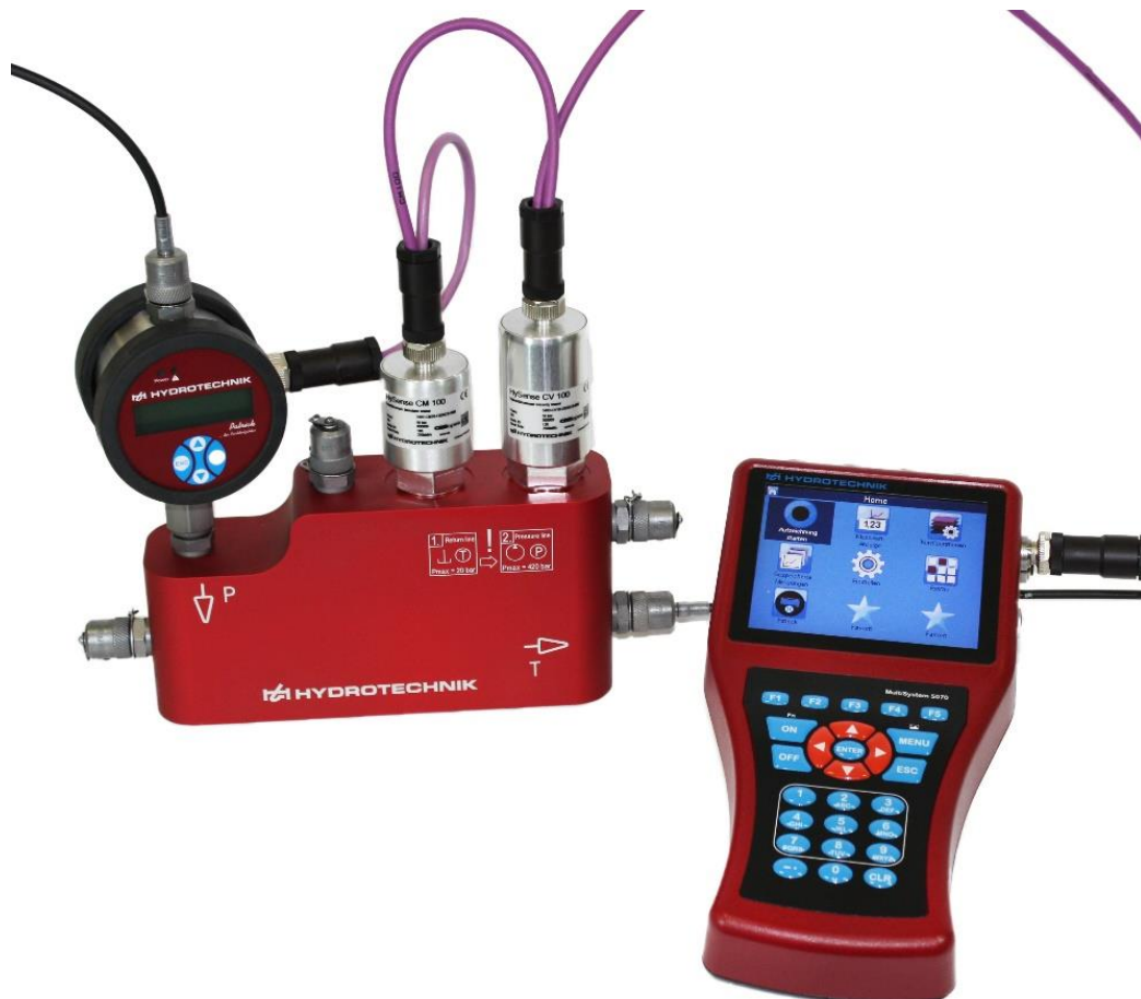
Figure 8: Service measuring kit connected to the MultiSystem 5070
